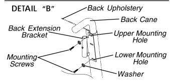
FIGURE 1 - INSTALLING THE BACK EXTENSION BRACKETS
